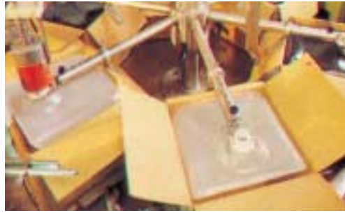
The Van Meurs Bag in Box filling machine. The simplicity of this unit almost eliminates operator error.
